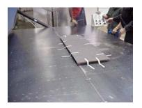
7. A silicone blanket is used as the diaphragm during this process. A thermocouple is used to record the temperature. The thermocouple is placed "in a pocket" on the blanket with a setpoint of 230°F (110°C). Correlation experiments have been performed to verify the temperature reading at this location relates to the actual glue line temperature. The Schneller HA211 adhesive system requires a temperature of 212°F (100°C), as measured at the glue line, to fully activate.
