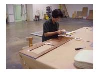
4. The mold/support tool for a 757 dado panel is simple since this dado panel is a relatively flat panel. Spacers are added to the backside of the dado to ensure the panel is not damaged during the application process.
