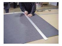
6. The mold is placed on the vacuum table (in an actual production scale set-up, more than one dado panel is recovered during one cycle). The decorative is attached to the dado panel to ensure the alignment is correct and remains correct during the application process. As shown below, this can be done with a heat resistant tape (or using a heat gun).
