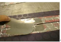
After trimming all of the seams, the material may be cut to the final size and shape.
