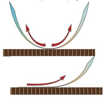
6. During the application process, it is important to "suspend" the material away from the panel when using a contact adhesive system. Typically, it is not possible to reposition the decorative laminate after the bond has set.
